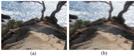
Fig. 4. (a) Progressive frame from a test sequence. (b) Same frame of the interlaced version of the video sequence.
